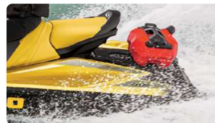
Swim Platform with Integrated LinQ System Exclusive quick-attach system on a large swim platform that allows for easy installation of storage accessories.
