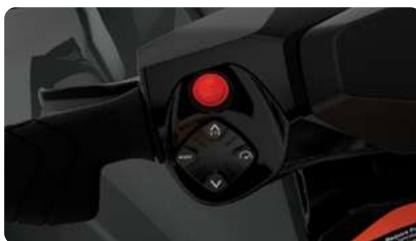
VTS™ (Variable Trim System) Provides handlebar-activated settings so riders can easily find the ideal trim for varying conditions.
